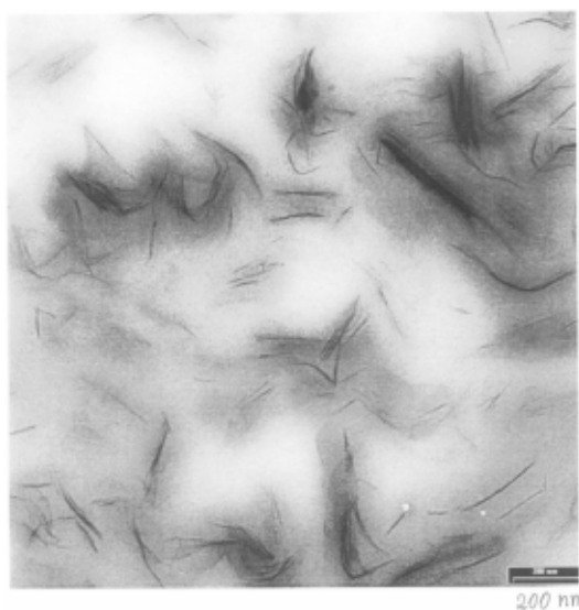
Fig. 4 Parallel cut of PP – Somasif ME 100 nanocomposite fibres
